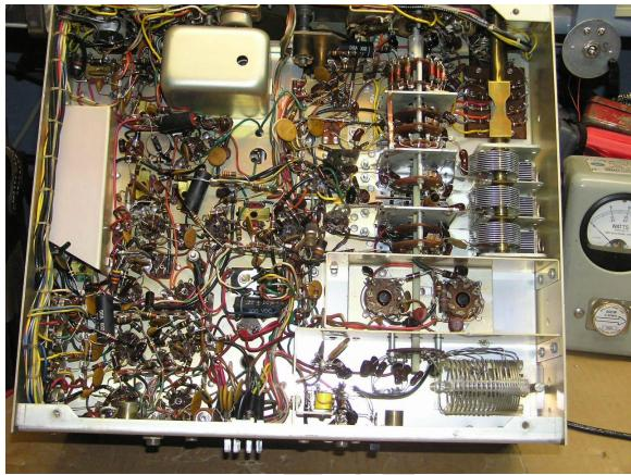
At this point I could not stand it, I had to see if it worked even with the bad tube socket. The relay problem doesn't impact normal operation of the rig. Upon power up there was no TX or RX. I quickly located the problem, no carrier osc, no plate voltage on V10. T4 open, I discovered the slug was frozen. At that point I had a hunch about what had happened. A prior owner tried to adjust the slug and had spun the form in the base. Inspection confirmed this as well as a broken form.
