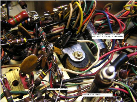
I had a T4 in a parts rig, replaced it and the rig actually worked. The receiver actually met factory specs but was not up to standard performance. The transmitter worked, but max output with a new matched pair of finals was 40 watts. So now its power down and start replacing wires, resistors, capacitors, relays and tube sockets. I got very busy in the shop so it went on the shelf..........
